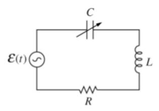
38. An AC circuit consists of the elements shown above, with R = 10,000 ohms, L = 25 millihenries, and C an adjustable capacitance. The AC voltage generator supplies a signal with an amplitude of 40 volts and angular frequency of 1,000 radians per second. For what value of C is the amplitude of the current maximized?
