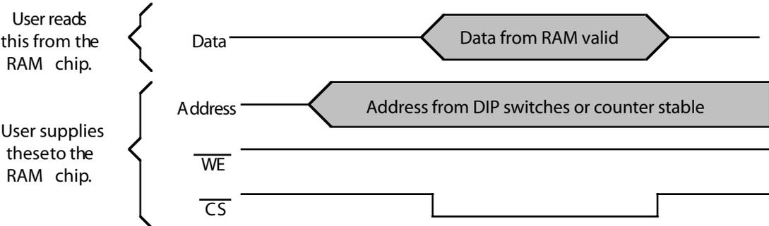
Figure 2: READ cycle timing diagram.
