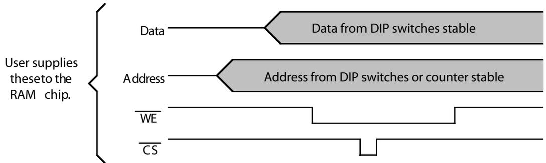
Figure 1: WRITE cycle timing diagram.
